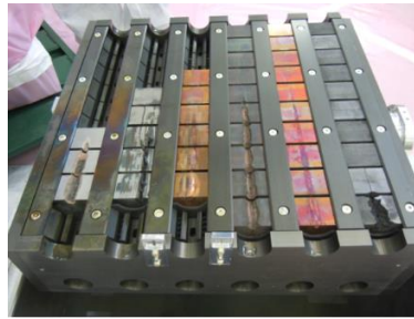
Figure 12 Results from HiRadMat's 2012 experiment on different material specimens' response under high-energy, high-intensity beams (From left to right: Inermet 180, molybdenum, Glidcop, molybdenum-copper-diamond, copper-diamond, molybdenum-graphite (three different grades))
